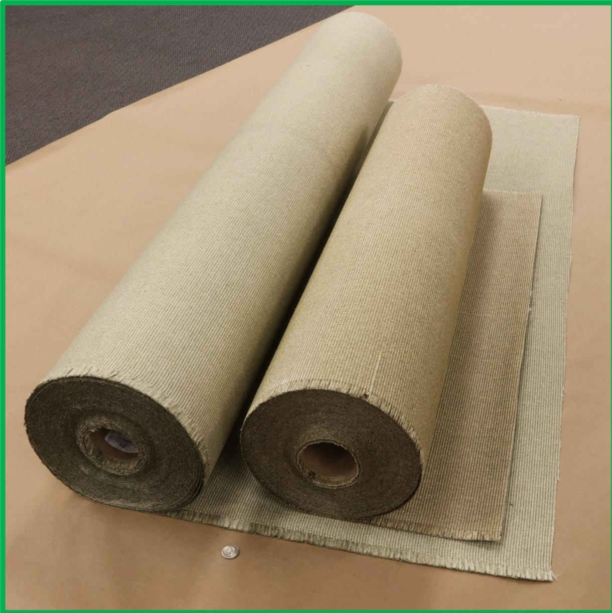
Manufactured of E-glass yarns, woven, and then immersed in a vermiculite dispersion to add thermal performance and additional abrasion resistance, this fabric has a 1500°F / 815°C continuous rating while providing high insulation value & excellent personnel protection. The polymer additive in the vermiculite dispersion provides a binding agent to make the fabric stiffer, easier to cut and handle, and provides anti-fray properties.
